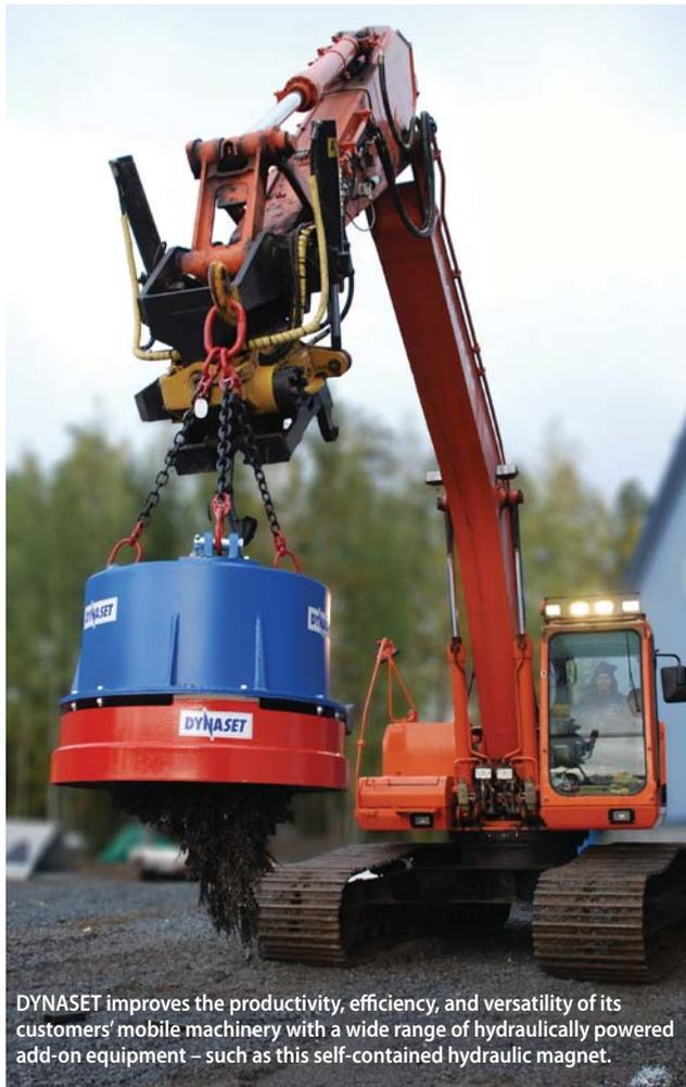
DYNASET improves the productivity, efficiency, and versatility of its customers' mobile machinery with a wide range of hydraulically powered add-on equipment – such as this self-contained hydraulic magnet.
